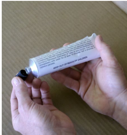
(3) Using the reverse side of the cap, puncture the foil seal in tip of the tube.
