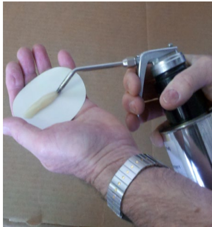
(3) Activate the trigger on the pump several times to prime the pump.
