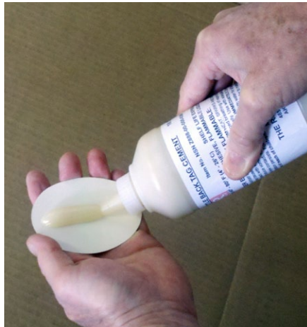
(3) Apply adhesive to back of tag to simulate a 1/4" bead across the middle of the tag.
