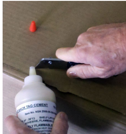
(2) Using a utility knife, cut the tip of Yorker Spout to the desired diameter.
