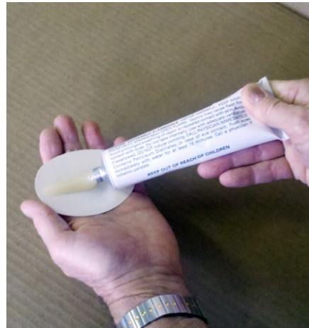
(4) Apply a bead across the middle of the back of the tag (approx. 1/4" diameter).
